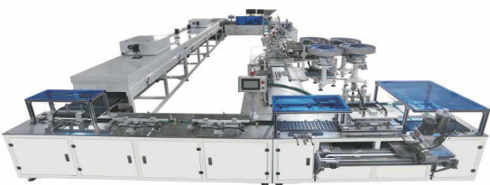
Fully automatic assembly and packing machine for blood collection needles
