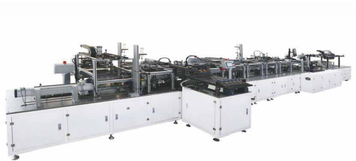
Fully automatic assembly and packing machine for scalp vein set
